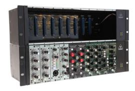
The Deca-Dent is powered externally by a switch mode power supply that can operate in any country without having to change any voltage settings. The power supply provides 32 Volts via a +/- 16V rails and a separate +48V rail for phantom power. Each slot get's the full 130mA requirements when under a full 10 unit load.
