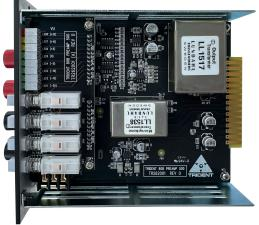
The **80B MIC PRE** amplifier is of a unique design that is able to handle signal levels from -60dBu to as high as +15dBu without the use of a separate pad switch. Even though such a wide range of signal levels is accommodated, adjustment of the gain is extremely smooth, particularly at the high signal levels where other designs tend to have a cramped level adjustment at the end of the control.
