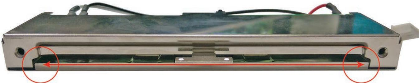
**Figure 1:** Start by blowing one end, and then the other. There is usually dust or debris in the fader that will come out easily, and this usually would be all that is needed in terms of cleaning. Move the fader carriage to one end and blow air into the slot aiming away from the carriage so that dust can escape through the slot. Then move the carriage to the opposite end and blow air aiming the opposite way.
