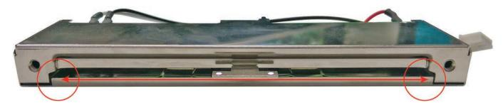
**Figure 1:** Start by blowing one end, and then the other. There is usually dust or debris in the fader that will come out easily, and this usually would be all that is needed in terms of cleaning. Move the fader carriage to one end and blow air into the slot aiming away from the carriage so that dust can escape through the slot. Then move the carriage to the opposite end and blow air aiming the opposite way.
